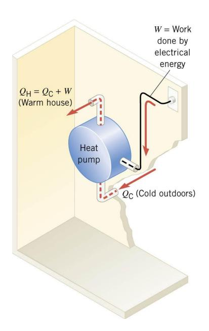
In a heat pump the cold reservoir is the wintry outdoors, and the hot reservoir is the inside of the house.
