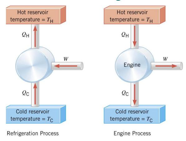
In the refrigeration process, work W is used to remove heat  $Q_{\rm C}$  from the cold reservoir and deposit heat  $Q_{\rm H}$  into the hot reservoir.
