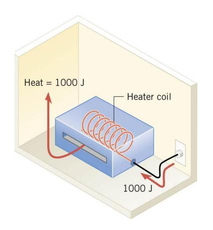
This conventional electric heating system is delivering 1000 J of heat to the living room.
