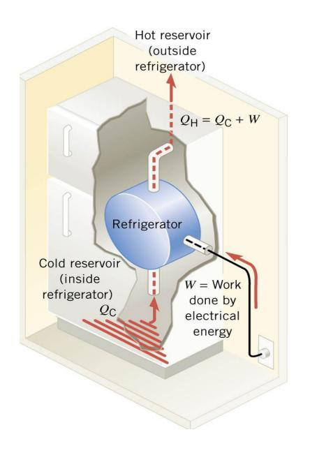
In a refrigerator, the interior of the unit is the cold reservoir, while the warmer exterior is the hot reservoir.
