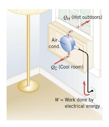
A window air conditioner removes heat from a room, which is the cold reservoir, and deposits heat outdoors, which is the hot reservoir.
