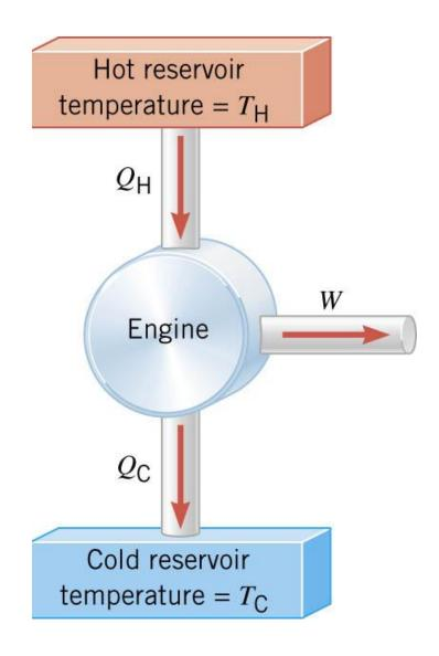
A Carnot engine is a reversible engine in which all input heat  $Q_{\rm H}$  originates from a hot reservoir at a single temperature  $T{\rm H}$ , and all rejected heat  $Q_{\rm C}$  goes into a cold reservoir at a single temperature  $T_{\rm C}$ . The work done by the engine is W.
