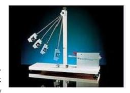
measuring how high the pendulum would swing, one could determine the initial velocity of the bullet. It's unclear why we stopped using real rifles. Today, the basic idea remains the same: a projectile is fired into a (hollow) pendulum bob and remains embedded in it.
